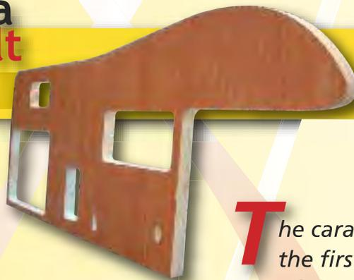
**T**he caravan industrial field was one of the first to understand main advantages of this bonding, for a higher quality level of external walls, making faster the production process. Since some years, the most important recreational vehicles producers are using wide OMMA Hot Melt rolls coaters (from 2.500 over 3.000mm), for this purpose. The experience acquired on this matter is also transferred to the narrower machines, in order to improve quality level and performances.
