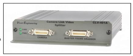
One frame grabber acts as master and provides control and communications to the camera. The second frame grabber receives camera video data only.
