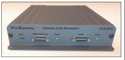
enhanced timing performance, bayer color support, and color bar & pseudo-random video patterns. Control is via an RS-232 port, USB, or frame grabber comm port. The CLS-222 also supports the AIA validation test pattern.
